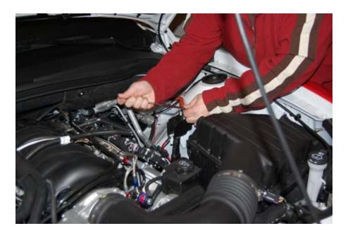
10. Route the red wire of the NX relay harness (AKA relay trigger wire) through the previously mentioned firewall grommet. Cover the wires with split loom and electrical tape for a clean factory look. Replace the engine cover and oil cap.
