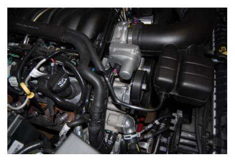
4. Apply a thin bead of silicone to the mounting flange of the throttle body.
