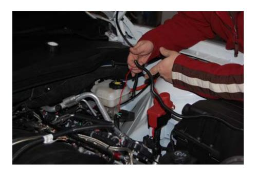
Attach the white wire of the NX relay harness to ground (optionally through a fuel pressure safety switch). Connect the black wire of the NX relay harness to the positive battery stud on the driver's side of the engine bay (we chose to install an optional fuse in this wire).
