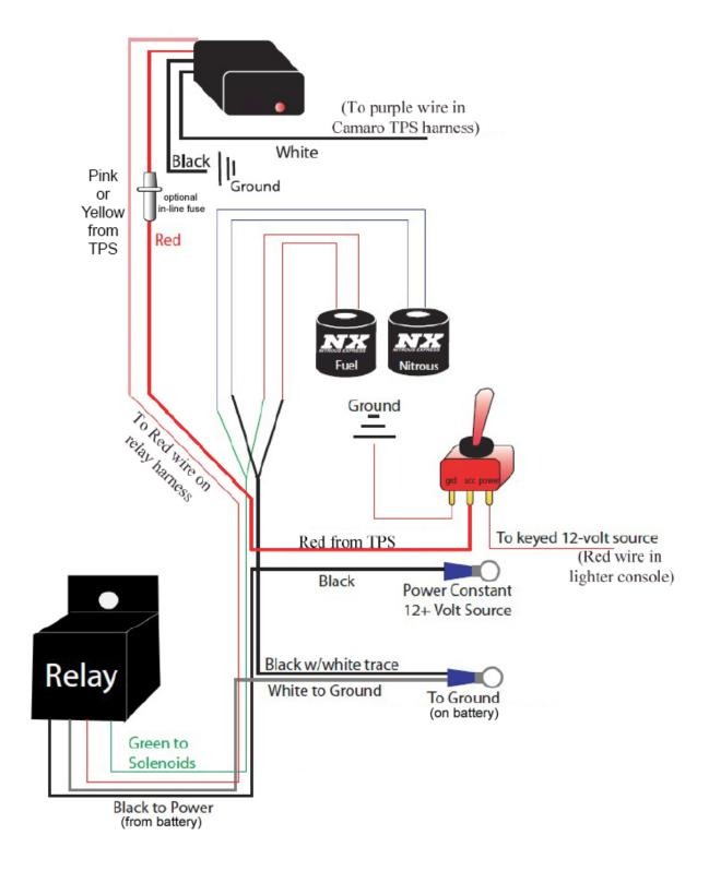
Attach the white wire of the TPS module wire to the purple wire of the Camaro throttle body harness (AKA TPS Wire). NOTE: The TPS module will be mounted inside, so you should route the white wire from the TPS module
