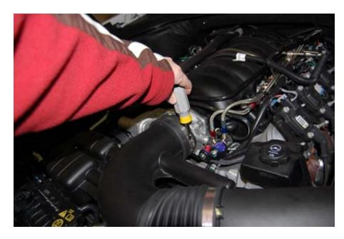
3. Unplug the harness from the throttle body and remove the four bolts that attach the throttle body to the intake manifold.
