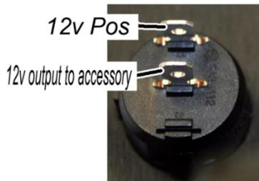
**On/Off Switch Wiring**
