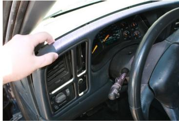
4. Once the dash is removed unclip the small storage compartment, this will be replaced with the switch panel.
