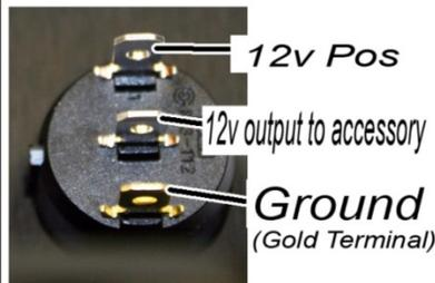
**Bottle Opener Switch Wiring**
