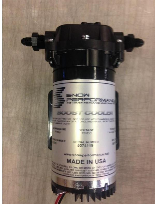
Step 2: Install the fluid pump with four (4) #8x1&1/2" screws and four (4) #8 washers (supplied) in desired mounting location.
