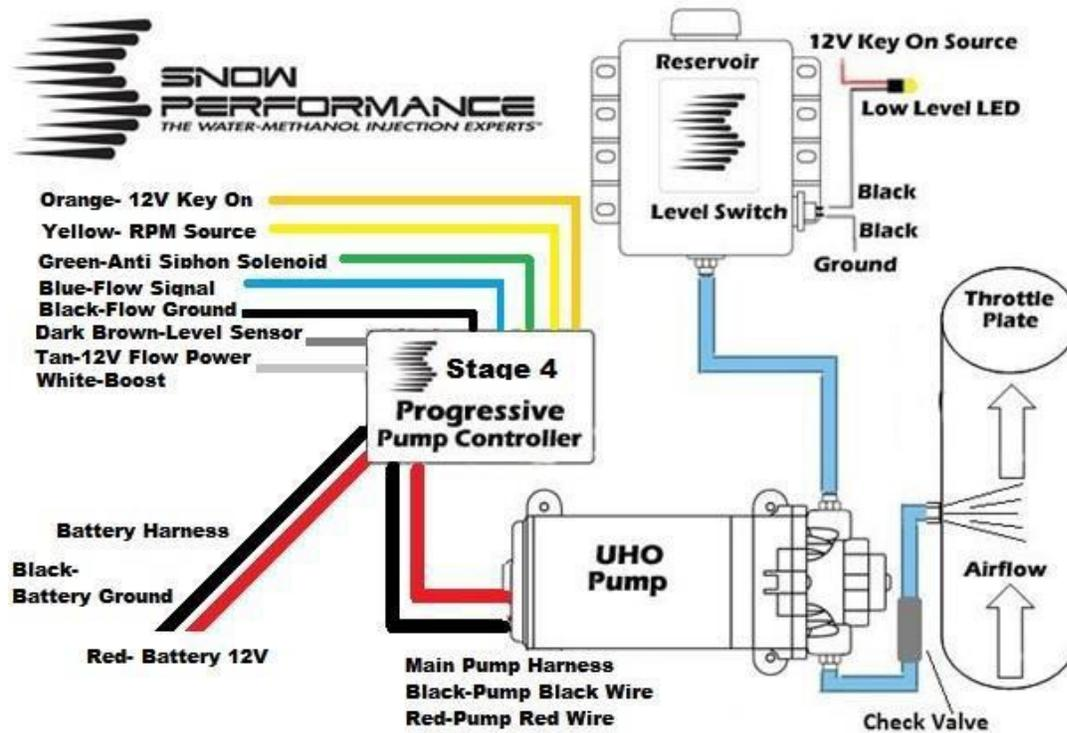
Step 1: Plug in the main wiring harness, main pump output harness and battery power harness into the Stage 4 control unit. Place controller in vehicle glove box or under passenger seat ensuring easy access. Run the wires of these harnesses through the fire wall of the vehicle and into the engine bay.
