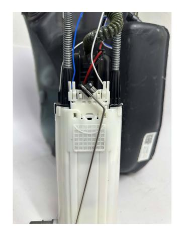
11. Now take your assembled Snow Performance Multi-Pump Fuel Hat assembly and remove two of the three fuel pump hangars. There are two screws per hangar, ensure that you do not lose these or the o-rings.
