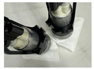
TIP: When installing the fuel pump hangars, ensure that the tabs around the pump bases "lock" together.
