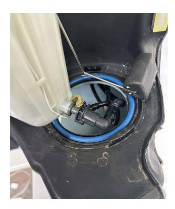
9. Remove the OEM pump assembly and safely drain and contain any residual fuel in the assembly. Inspect the large blue seal insuring it is not damaged or compromised.
