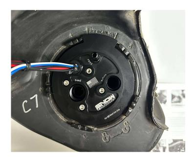
21. Reconnect the EVAP fitting to the port on top of the fuel hat. Using the proper tool and socket wrench, reinstall the lock ring.
