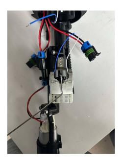
17. Tilt the assembly so the fuel level float fits into the tank. While holding the fuel hat slightly out of the tank, re-install the fuel pump hangars one at a time.
