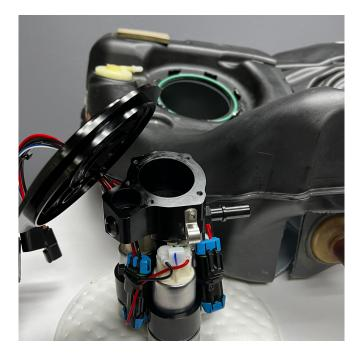
22. Carefully lower the fuel pump assembly. It is normal to have a slight interference with the fuel level sensor. When sliding the fuel level sensor past the tank opening, gently push the sensor inward. For proper orientation, reference the Snow Performance logo or the images that follow.
