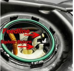
12. Remove the OEM pump assembly being sure not to damage the float arm. Safely drain and contain any residual fuel in the assembly. Inspect the large green seal insuring it is not damaged or compromised.
