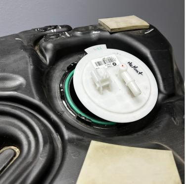
21. Unbolt the top of the new Multi-Pump Fuel Hat to give clearance for connecting the feed-line and siphon return.
