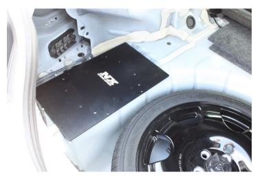
The Trunk Multi-Mount bracket can be used with one of multiple NX or Snow Performance accessories listed below:
