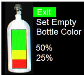
This is your Bottle Level Screen. Because EMPTY is subjective, different users will have different levels at which they consider the bottle to be empty. The gauge is programmed with a default empty level and may not accurately display the true level in your tank until you have calibrated it. This will be discussed at the end of the programming section.
