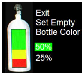
This is the Green to Yellow change point which is a visual aid on the main viewing screen. To change the %, push your control button in (the text will change to blue) and toggle up or down to change the value. If you hold the control button in the up or down position, the numbers will scroll. Once you have the % programmed for your needs, push the control button in to save it.
