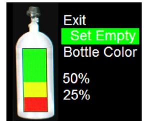
**Important:** Each time the gauge detects that your solenoids are activated, it begins to track your nitrous usage and will display an hourglass ICON. **DO NOT power off the gauge while the hourglass ICON is present.** Once the gauge detects that no further solenoid activity has occurred, it updates the usage log and turns off the ICON. At this point it is safe to power off the gauge. Failure to do this will impact the accuracy of the gauge.
