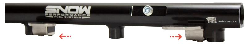
12. Plug any of the four 1/8" NPT ports on the rail you will not be using.
